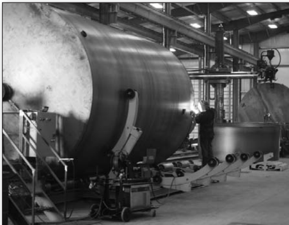
Oil Tank Production at Pro Tank Products
